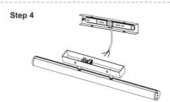
Remove the line pressing clip, connect the wires correspondingly.
